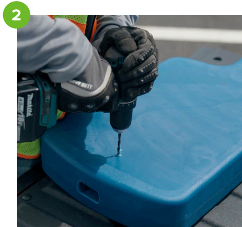
Using a drill and a 3/16" drill bit, drill holes where you marked.
