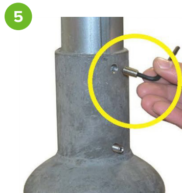
5 Using the cone point set screw and allen wrench, pierce the pipe with this set screw for post retention.
